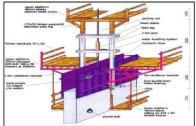
Fig 4 :- Components of Slip Formwork
